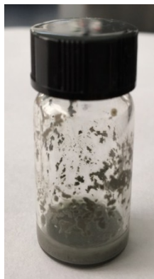
Figure S1. Photograph of the as-prepared AgNW-HPMC-Ink showing obvious aggregations of the AgNWs on the sidewalls of the container.
