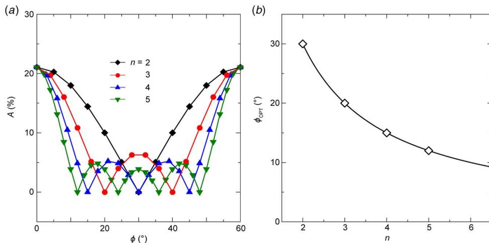
**Fig. 4 (a) Mechanical anisotropy degree in multilayer graphene as a function of  $\phi$ . (b) Optimal interlayer twist angle to minimize the mechanical anisotropy as a function of  $n$ .**
