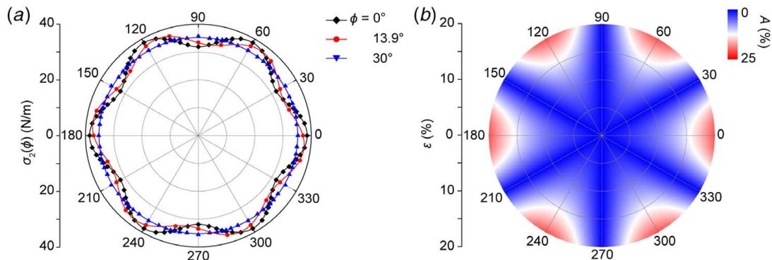
**Fig. 3** (a) Stress distribution of twisted bilayer graphene under tensile strain of 20% as a function of  $\theta$ . The lines are from theoretical predictions and the dots are from direct simulations. (b) The mechanical anisotropy degree of bilayer graphene as a function of  $\epsilon$  and  $\phi$ .
