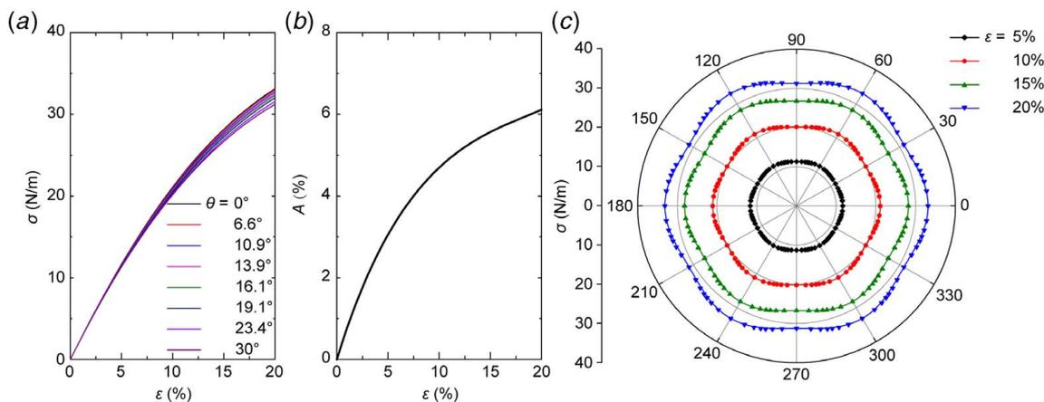
**Fig. 5 (a) Stress–strain curves of  $h$ -BN oriented along different directions subjected to tensile loads. (b) Mechanical anisotropy of  $h$ -BN as a function of tensile strain (Eq. (1)). (c) Orientation-dependent mechanical responses of  $h$ -BN subjected to different magnitude of tensile strain as a function of  $\theta$ . The dots and lines are from the simulations and predictions, respectively.**
