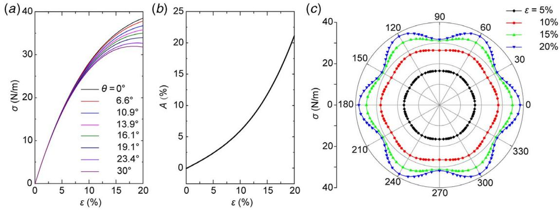
**Fig. 2** (a) Stress–strain curves of graphene oriented along different directions subjected to tensile loads. (b) Mechanical anisotropy of graphene as a function of tensile strain (Eq. (1)). (c) Orientation-dependent mechanical responses of graphene subjected to different magnitude of tensile strain as a function of  $\theta$ . The dots and lines are from the simulations and predictions, respectively.
