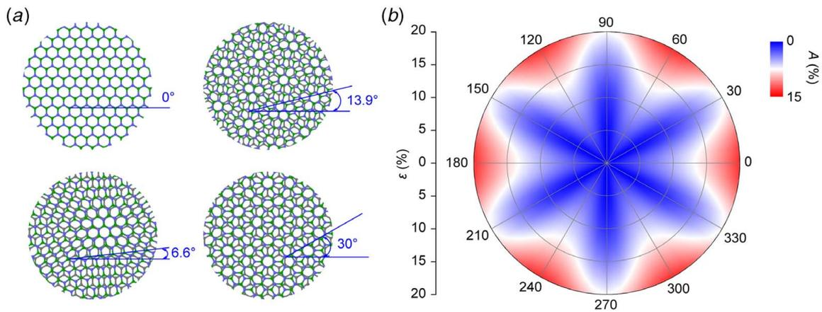
**Fig. 6 (a) Typical Moiré Patterns in bilayer graphene/h-BN heterojunctions with  $\phi$  of 0 deg, 6.6 deg, 13.9 deg, and 30 deg, respectively. (b) The mechanical anisotropy degree of bilayer graphene/h-BN heterojunctions as a function of  $\varepsilon$  and  $\phi$ .**
